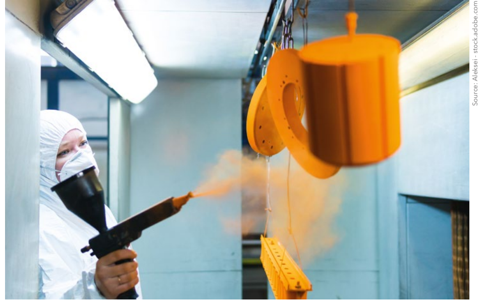
③ Powder coatings can be applied to a variety of products and substrates.
